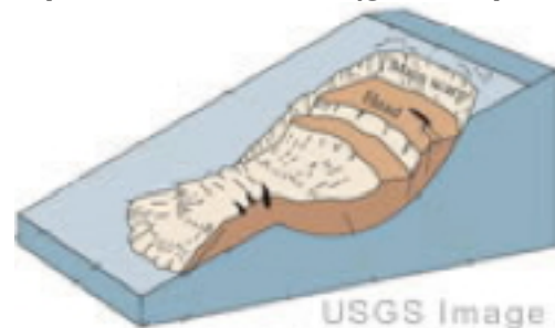
Fig. 16 Below: Undercut river banks, and river bank collapses, are not unusual but rather normal for rivers and inlets. Image shows collapse and full 'TOE' (geomorphology term).
